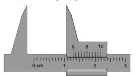
Look at the picture of the caliper. It marks 1,28 cm. To know it, you have to look at the 0 in the mobile scale (the superior one) which is between 1,2 and 1,3, but closer to 1,3. Now, look for the marks in both scales, superior and inferior, that are in the same position. In this case, is the eighth mark in the superior scale, so the value is 1,28 cm.
